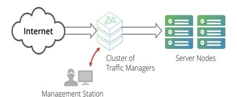
A cluster of Traffic Managers is typically managed through the web-based administration user interface (Admin UI) on one of the cluster members. The Traffic Manager's REST API provides an alternative means to remotely administer, configure, and monitor a Traffic Manager cluster.
